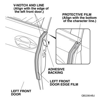
8. Align the center line on the left front door edge film with the edge of the left front door. While applying light pressure, carefully remove the adhesive backing.
