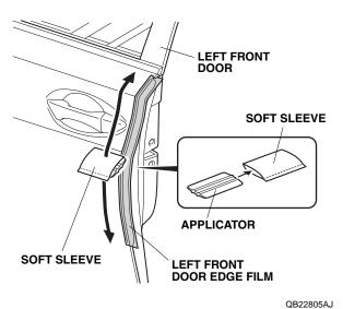
10. Slowly remove the protective film from the left front door edge film.
