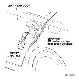
14. Open the left rear door. Peel back about 50 mm (2.0 in.) of adhesive backing from the left rear door edge film. Align the V-notch on the left rear door edge film with the left rear door as shown.
