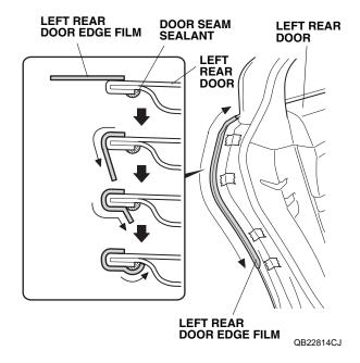
19. Using a shop towel, wipe the excess 3M protective tape application solution from the left rear door edge film. Allow the left rear door edge film to dry thoroughly.
